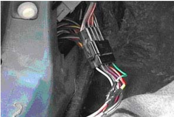
Figure 2 (VSS signals behind driver's kick panel)
